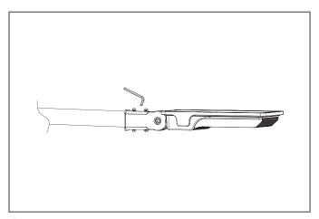
② Install the hole lamp on the pole and tighten four M8 screws.
