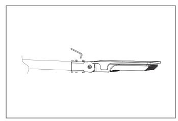
② Install the hole lamp on the pole and tighten four M8 screws.
