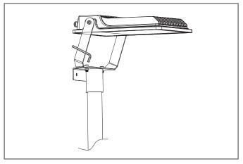
① Install the hole lamp on the pole and tighten four M8 screws.
